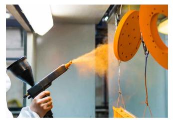
Chrome free coating for Aluminium and Iron Phosphate for Ferrous and Galvanized steel products. In all there are 9 stages to Intercare's pretreatment for Powder Coating.
